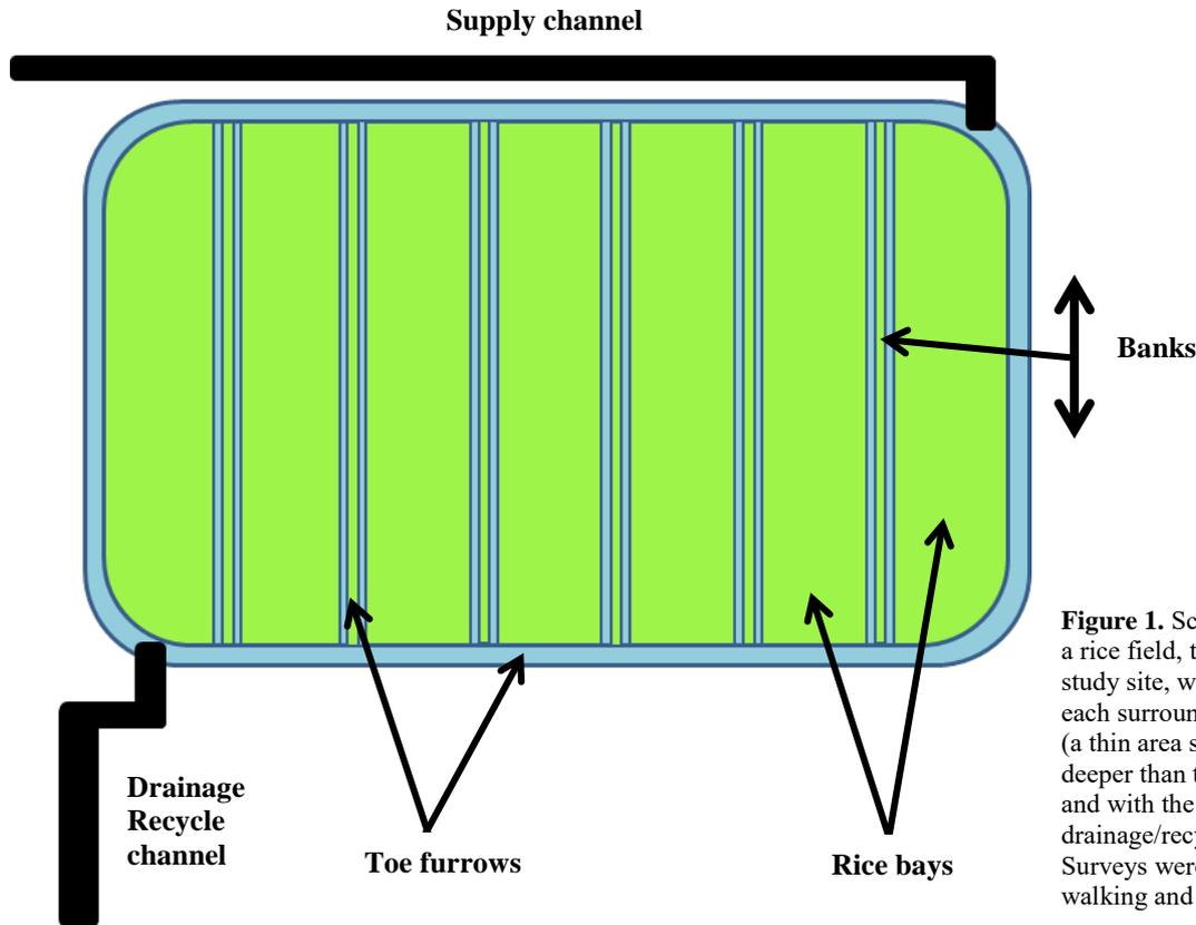
**Figure 1.** Schematic diagram of a rice field, typical of a single study site, with seven rice bays, each surrounded by toe furrows (a thin area surrounding the bay, deeper than the crop) and banks, and with the supply and drainage/recycle channels. Surveys were conducted by walking and driving along banks.
